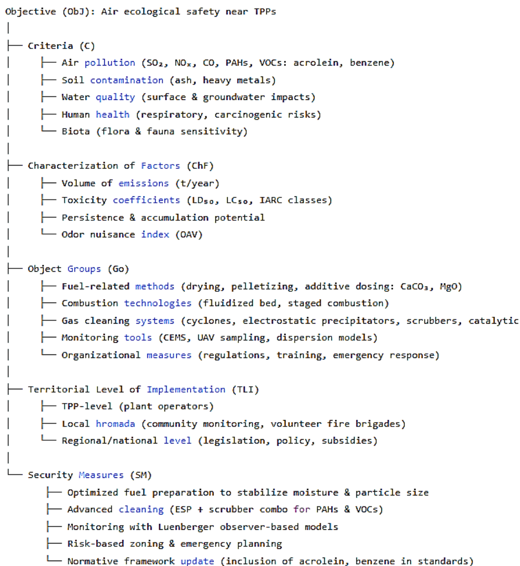
Figure 2 – Scheme of hierarchical decomposition (AHP-based model)
